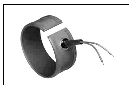
Fig. 5 – Leads exit at right angle to sheath 5/8” from gap. 12” lead wire in 3” long sleeving is standard. Specify alternate position.
