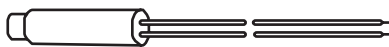
TYPE L - PTFE Lead wire 36" standard Ground lead is optional on all terminations
