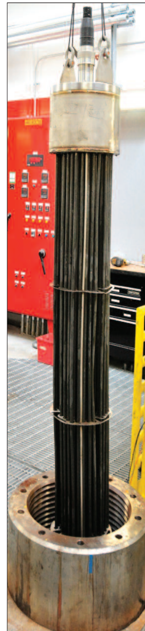
Subsea heater - 5000V, 3500m depth
