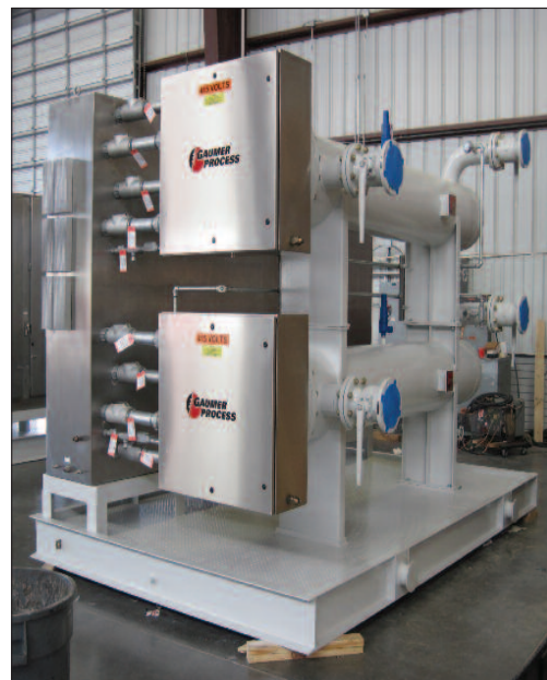
Diesel fuel oil heaters
