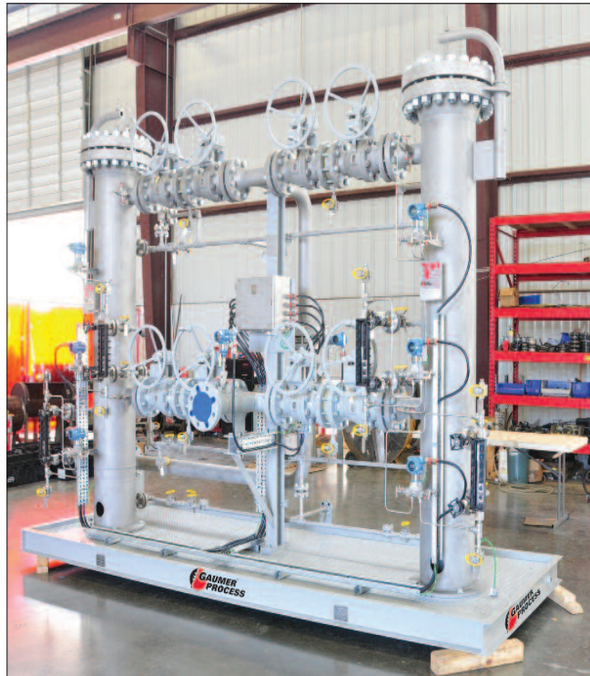
Fuel gas, double block & bleed
