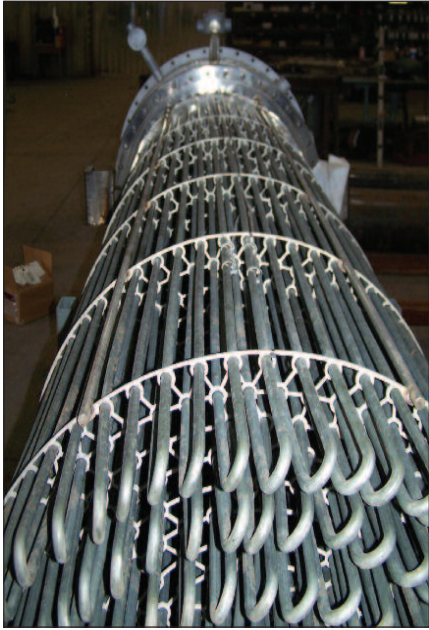
36" heater for oxygen service
