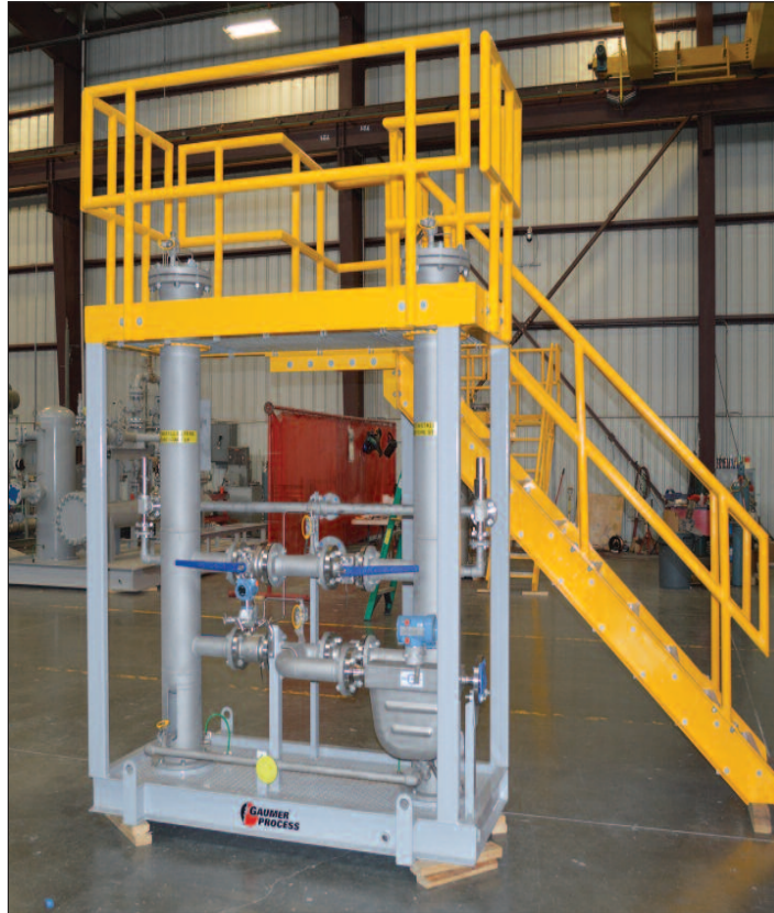
Staircase to Australian standards
