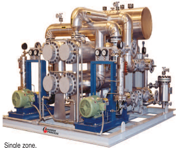
Single zone, 100% SCR for extruder plant
