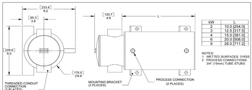
CONNECTIONS: 1/2 inch (12mm) or 3/4 inch (19mm) tube connections (custom connections available).
