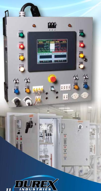
pre-wired and tested at the factory and come with a set of drawings including schematics and I&M manuals. Standard panels include NEMA 12 enclosure, main power disconnect, process temperature controller, pilot lights, panel labels, primary and secondary fusing, and ventilation fan /filter (if required).
