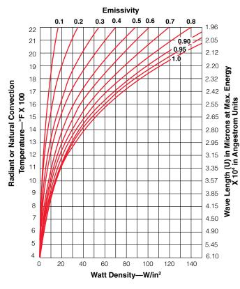
Determining MULTICELL Process Watt Density and Sheath Temperature: The process watt density is found on the W/in<sup>2</sup> scale (lower) at the intersection of the process temperature value (left temperature scale) and the 1.0 emissivity curve. The MULTICELL sheath temperature is found on the left temperature scale at the intersection of the heater emissivity curve (0.90) and the process watt density added to the heater design watt density (lower W/in<sup>2</sup> scale).
