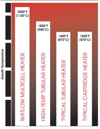
Engineered to handle applications that demand high temperatures, MULTICELL heaters from Watlow have a rugged construction that permits the heaters to survive in conditions that would normally be lethal to other heater types. These MULTICELL heaters have been engineered to achieve process temperatures up to 2050°F (1120°C).
