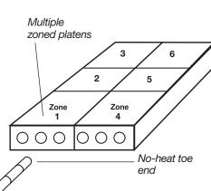
No-heat section designed for longer element life
